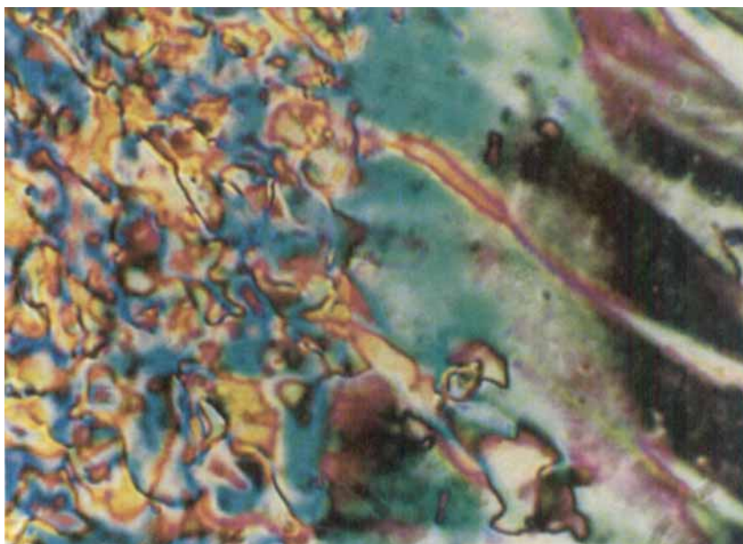
Figure 2. Optical textures of the N phase of compound IA ( n = 10 ) at 185^\circ\text{C} .
